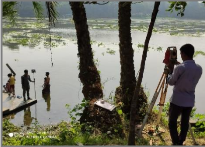
Total Station Survey going on for River Front Development Action Plan for Narail Municipality
